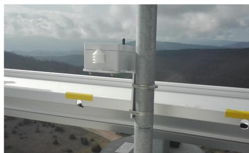
Fig. 2 – Example of smart-sensing device installed on the met mast that supports the wind sensors of the turbine
