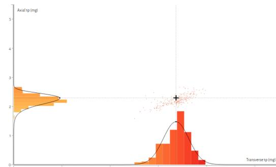
Fig. 3 – Representation of the distribution of the measured 1p acceleration peaks on the axial and transverse axes. The coordinates of the represented cross correspond to status of the rotor balance of the wind turbine.
