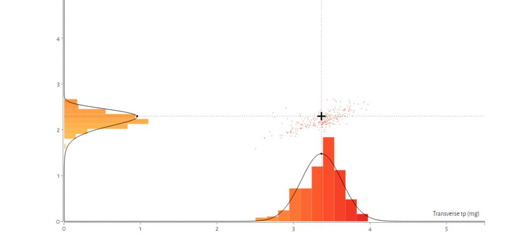
Fig. 3 – Representation of the distribution of the measured 1p acceleration peaks on the axial and transverse axes. The coordinates of the represented cross correspond to status of the rotor balance of the wind turbine.
