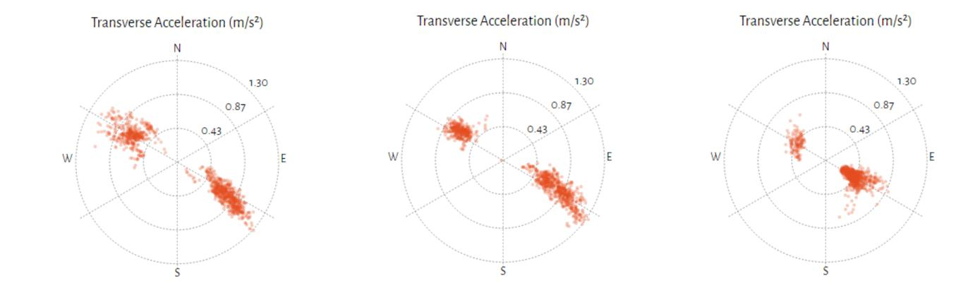
Fig. 4 – Measured vibration roses from 3 of the equipped wind turbines. A curtailment is applied in the NW wind sector in all 3 turbines to reduce the structure fatigue. Results show that the curtailment is unnecessary for 3<sup>rd</sup> turbine as it presents lower vibration levels in this wind sector.
