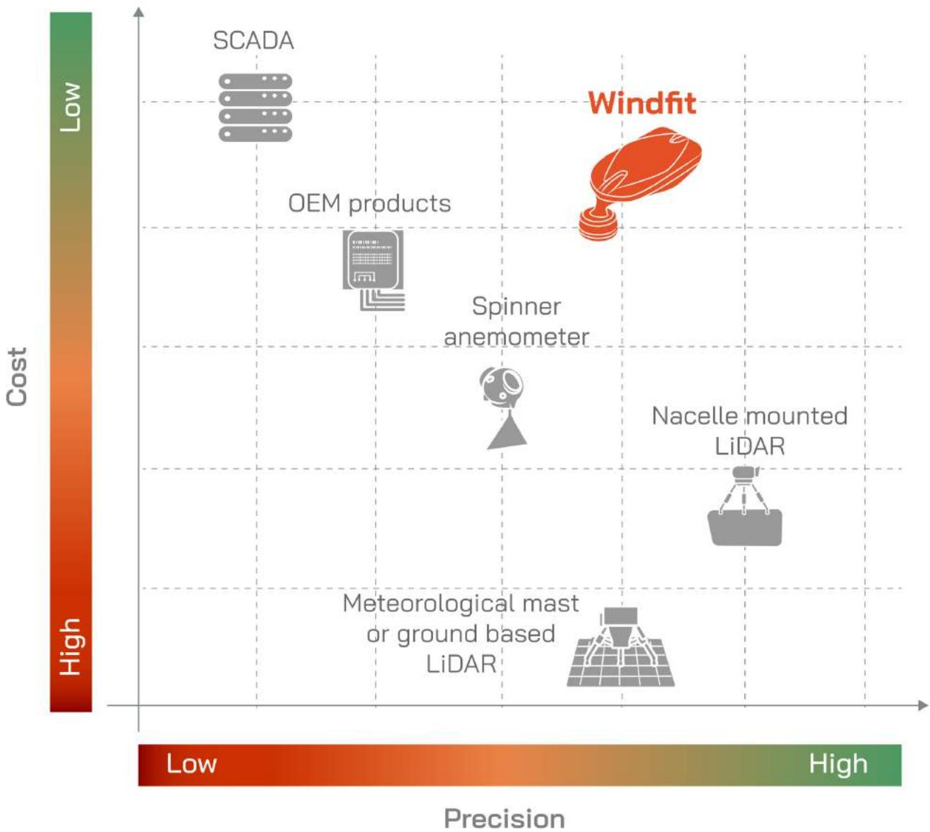
**FIGURE 7. COST VS PRECISION COMPARISON OF TRADITIONAL VS NOVEL TECHNIQUE.**
