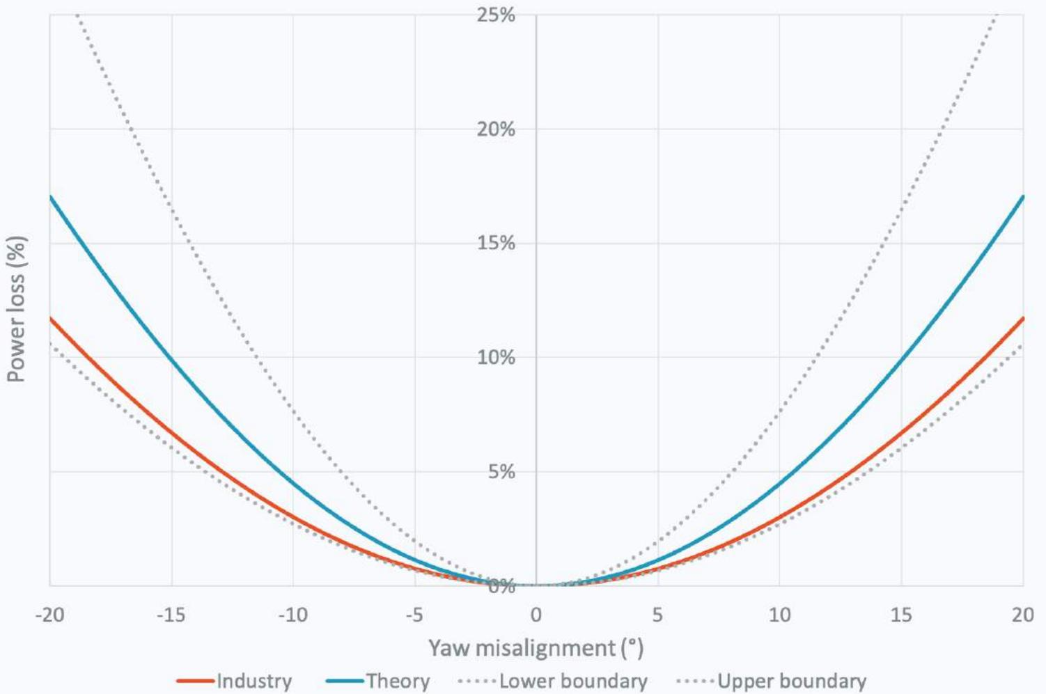
**FIGURE 4. POWER LOSS AS A FUNCTION OF YAW MISALIGNMENT FOR DIFFERENT CASES.**
