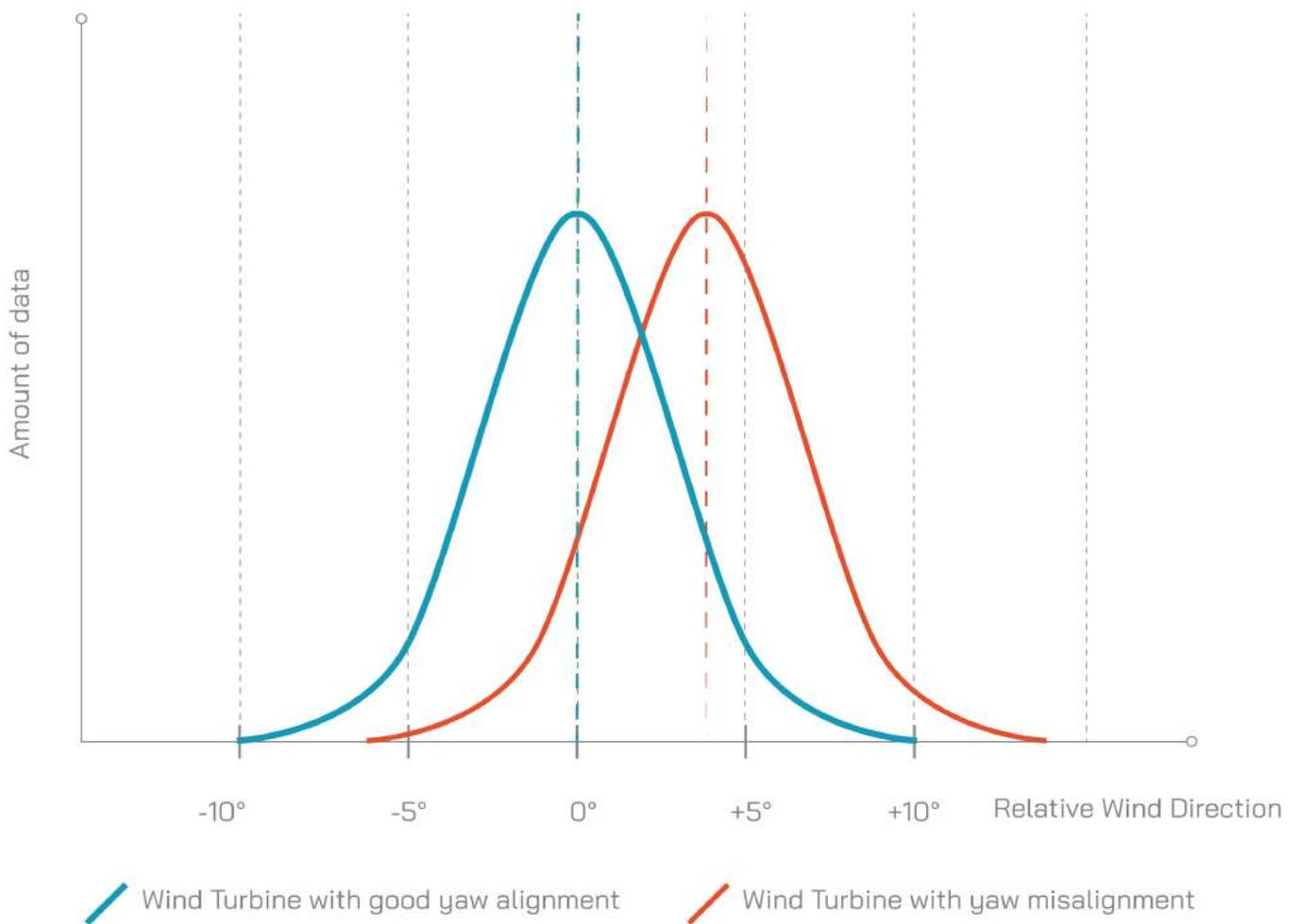
**FIGURE 3. TURBINES WITH DIFFERENT YAW MISALIGNMENTS.**
