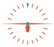
The yaw system is the mechanism all modern turbines have to handle direction changes on the wind. As winds are not constant by nature, wind turbines always need to face the wind to keep generating electricity. In order to do that, turbines are equipped with one or multiple wind sensors that measure the wind direction.
