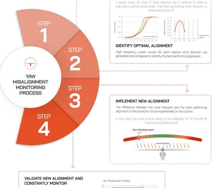
As soon as the correction is implemented, measurements will allow to confirm the new alignment and the increase in performance.
