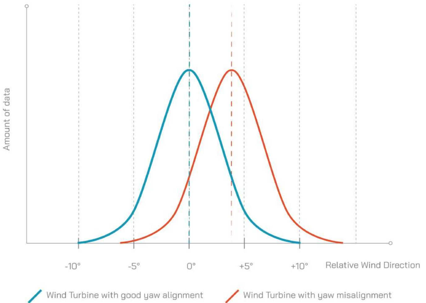
**FIGURE 3. TURBINES WITH DIFFERENT YAW MISALIGNMENTS.**
